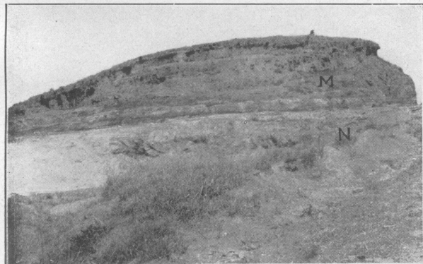
Fig. 3. An artificial cliff of the lowest part of the Manda Group (M), conformably overlying the Nanaura Sandstone (N); the slope from back to front is the stratigraphical boundary plane; half middle way from the Nanaura Mine to the Kachidachi Mine.
