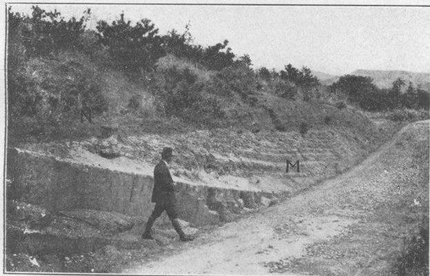
Fig. 3. East of Nobara Village, on the road, thin bedded alternation of sandstone and sandy shale of the Manda Group (M) unconformably overlaid by sand with gravels of the Nobara Beds (N).
